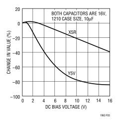
Figure 3. Ceramic Capacitor DC Bias Characteristics
