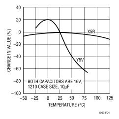
Figure 4. Ceramic Capacitor Temperature Characteristics
