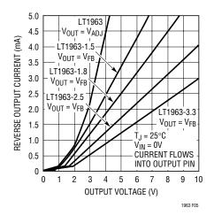
Figure 5. Reverse Output Current
