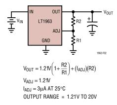
Figure 2. Adjustable Operation
